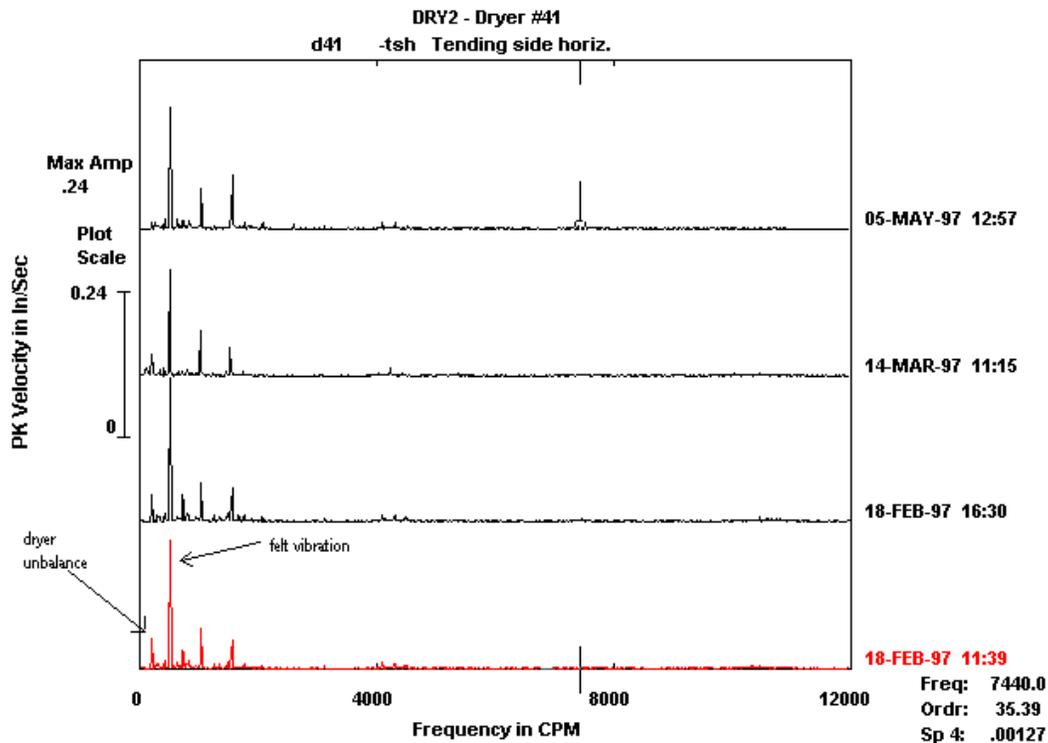
Fig 9 • Vibration Force due to Felt Roll Unbalance
