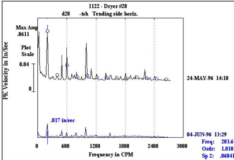
Fig 7 • 1<sup>st</sup> Field Balance Attempt (Before and After Single Run Balance)
